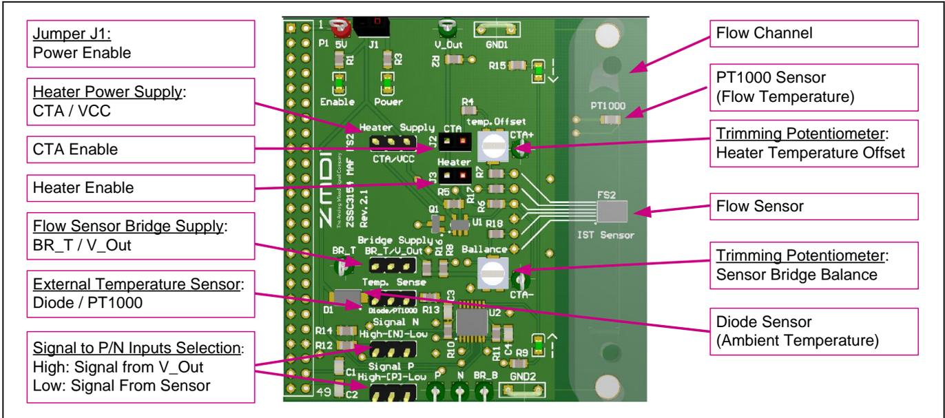
**Figure 3.2 FS2 Flow Sensor Layout**
