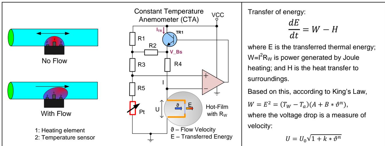
The air density can vary, which changes the thermal capacity of the air. The density is function of the ambient temperature, altitude, and pressure, which makes mass flow meters more appropriate for determining the quantity of the air.
